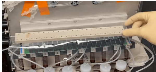
Figure 6-2: Aligning new membrane — channels facing downward
