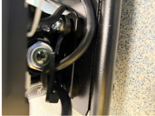
Figure A-2: Attaching muffler to exhaust port
