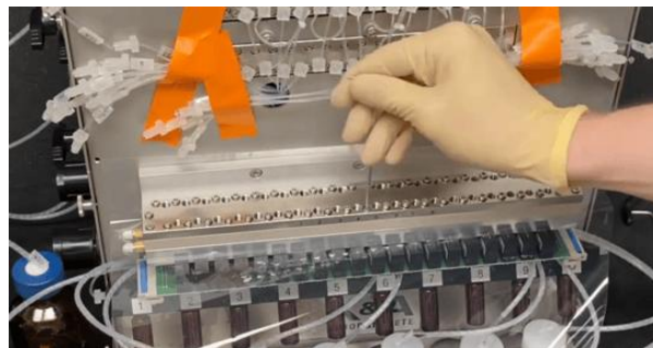
Figure 6-3: Inspecting luer fittings under columns
