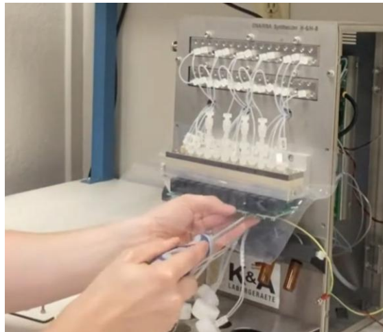
Figure 7-1: Carefully removing the electronic board
