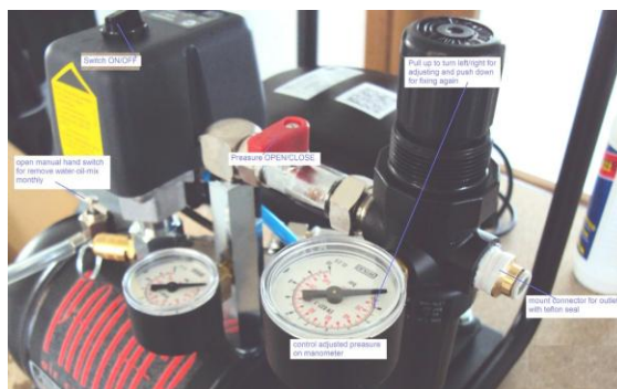
Figure A-3: Adjusting compressor output pressure
