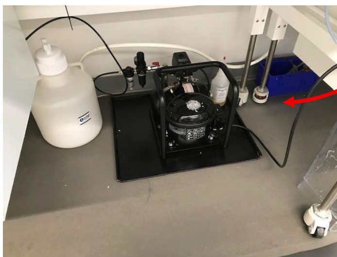
Waste and Air Compressor below the synthesizer
